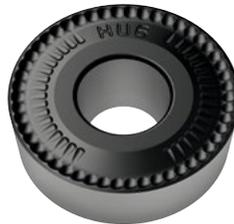
The circumference-sintered Tiger-tec® Silver insert with new HU6 geometry has been specially developed for the medium and heavy roughing of solid wheels and forged parts. A robust and powerful cutting tool with special chip grooves for ideal chip formation and a tool life that is up to 40 percent longer.
