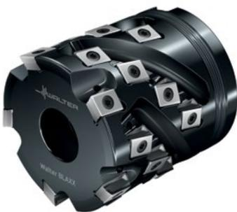
Equipped with four-edged, tangential Tiger-tec® Silver indexable inserts, the Walter BLAXX porcupine cutter is impressive thanks to its high metal removal rate and almost step-free contours. For even greater process reliability, each cutting edge has its own internal coolant supply.
