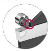
Existing grooving insert: The low chip shoulder makes the chip longer, meaning that it partially rubs against the top clamp.
